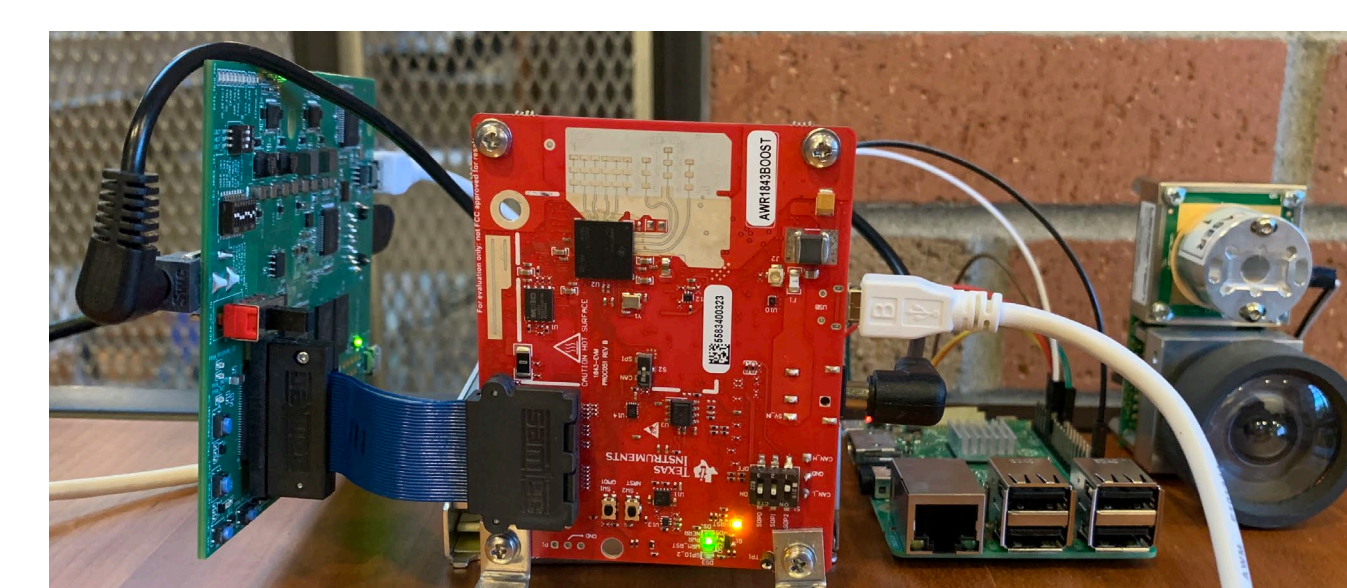
Figure 5: R-Pi connected to the LiDAR module as well as the radar module. Currently, the platform only supports triggering of a single sensor and the R-Pi can be switched over to trigger either of the module.
